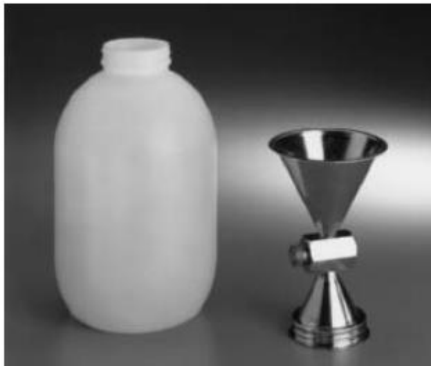
Figure 4.16 Plastic jar and the metal cone for the sand cone device (Note: The jar is filled with Ottawa sand.) (Courtesy of Braja Das)
