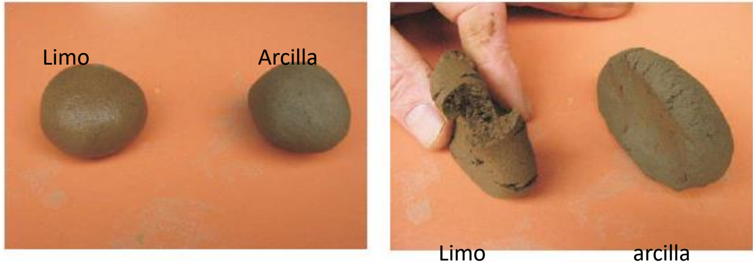
Figure 4.16 Cohesion of fine soils. The silt on the left breaks and starts to crumble, whereas the clay on the right deforms without rupture.
