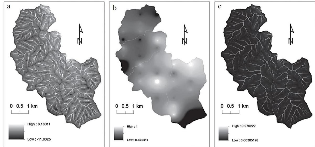
Figure 2. The predicted maps of (a) index of connectivity IC, (b) the maximum theoretical SDR coefficient  $SDR_{max}$  and (c) SDR variability within the study area. The IC and SDR maps in this figure were selected for spatial variability in 2007. Catchment boundaries are depicted in Figure 1
