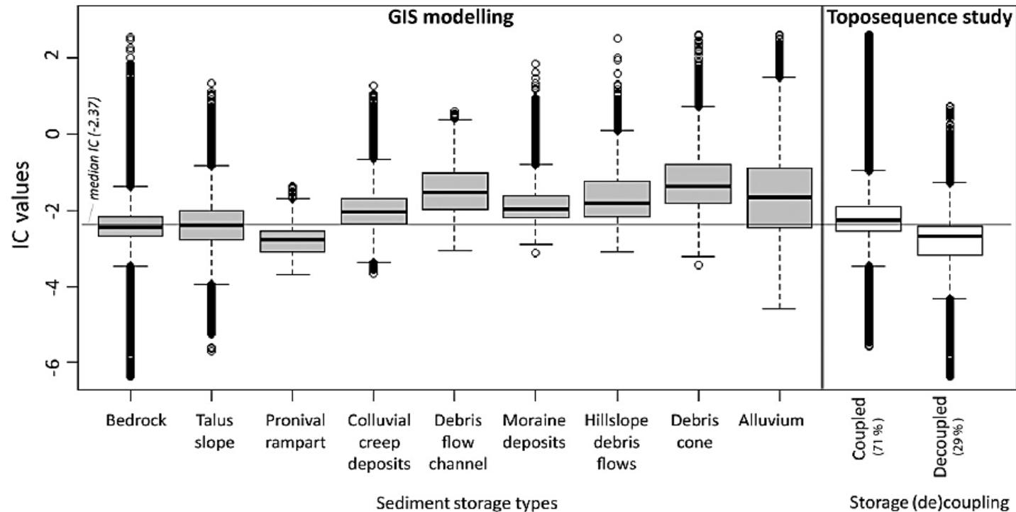
**Fig. 10.** IC values of sediment storage types in Val Mütschans and comparison between the modelling results (grey boxplots, left-hand side) and the field-based mapping results of the toposquence study (white boxplots right-hand side). Around 35% of the basin surface, which has been qualitatively classified as being decoupled, is related to IC values higher than the basin's median IC.
