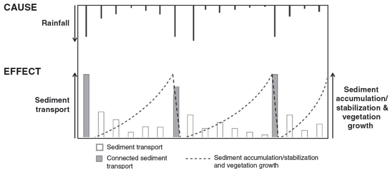
**Figure 4.** Diagram showing the effect of a major, infrequent event followed by low magnitude, high frequency events, which tend to decrease in magnitude over time as vegetation stabilizes hillslopes and river banks, as well as removing water from sediment transport via transpiration. This pattern continues until another high magnitude event occurs, leading to some form of resetting of the system.
