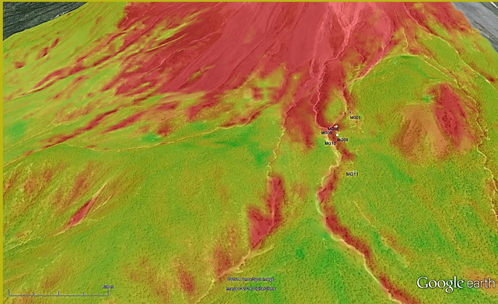
Connectivity may help understanding the dynamic of lateral hydrologic contributions that trigger or remobilize the lahars at the beginning of the rain season, when the soil is hydrophobic (Capra , Borselli et al. 2010).
