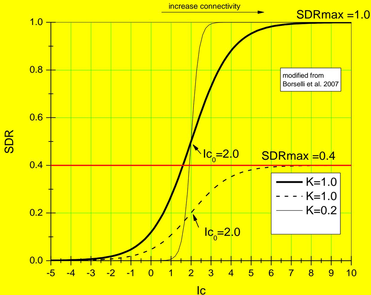
**Implementation of  $SDR = f(\text{conn. Index})$  For 4 types of connectivity indexes (including IC...) and optimization of parameters ( $Ic_0$  and  $k$ ) by Observed SSY at a series of Gauging stations**
