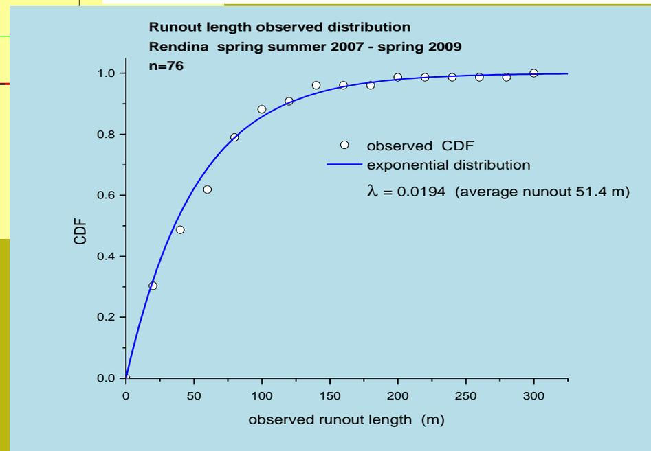
**Exponential probability distribution function depends from the average runout length  $L_r$  (measured) and the local site  $D_{dn}$  distance to a sink**
