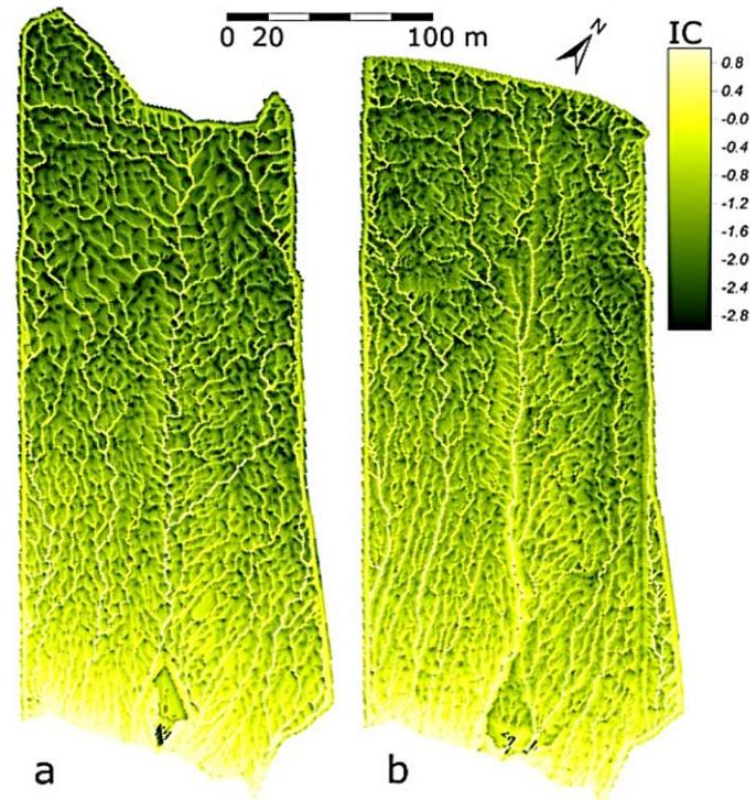
**Figure 13.** Spatial distribution of DEM cell values of the IC in the erosion-dominated area (as defined in Figure 3b), based on DEMs for (a) November 2005, and (b) March 2010. Grid cell size is 1 m by 1 m. Modification of the surface catchment area in autumn 2009 results in lower IC values in b).
