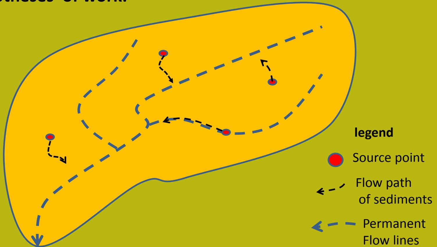
**Sediment travel time:** time  $\Delta T$ (s) required to move a given amount of sediments from a source point by a measured distance  $\Delta S$ (m) along a flow path. An average speed  $V$  can be calculated on the same **integrated interval of Time**  $\Delta T$ .
