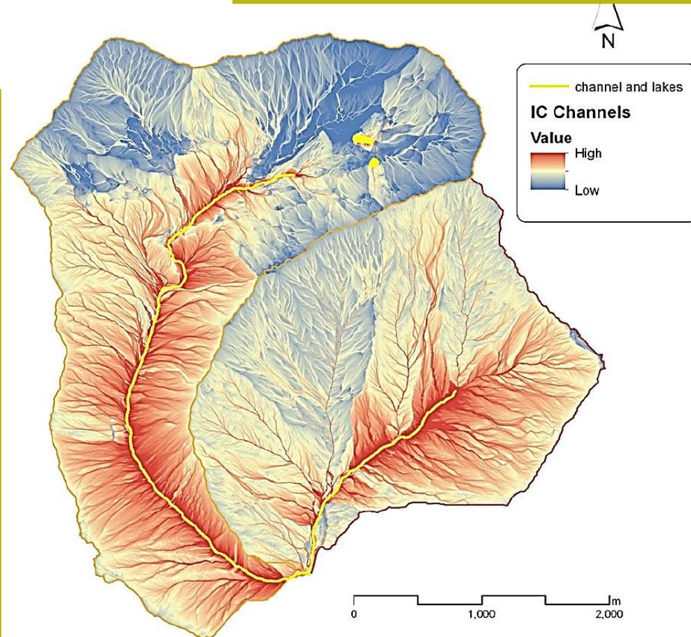
Fig. 5. IC channels map: index of connectivity IC computed with reference to main channels and lakes.
